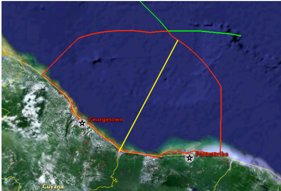
Figure 13. Division of the region shown in Figure 9 by the 28-degree line. The yellow line is a loxodrome with a bearing of 28 degrees. The green curves are extensions of the 200 nmi boundary.
