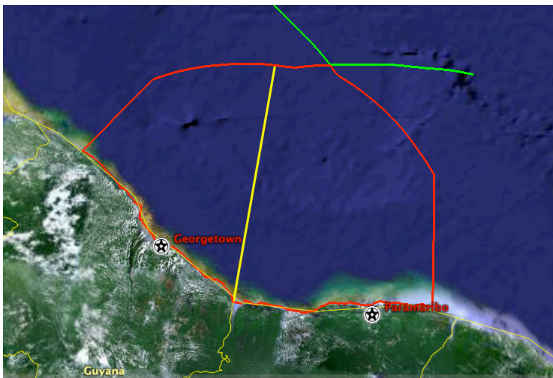
Figure 10. Division of the region shown in Figure 9 by the 10-degree line. The yellow line is a loxodrome with a bearing of 10 degrees. The green curves are extensions of the 200 nmi boundary.
